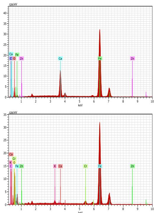
**Figure 7. EDAX analysis of rebar steel immersed in (a) SCPS in well water (blank) (b) SCPS in well water+ 250 ppm of Potassium dichromate + 50 ppm of Zn<sup>2+</sup>**
