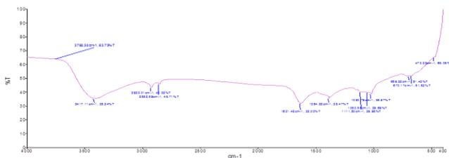
**Fig.5 (a): FTIR spectrum of Pure Potassium dichromate**
