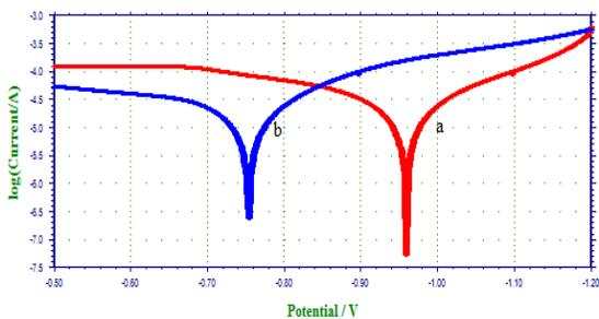
**Figure 1** Polarization curve of rebar steel immersed in SCPS prepared in well water a)SCPS b)SCPS + K<sub>2</sub>Cr<sub>2</sub>O<sub>7</sub> 250 ppm+ Zn<sup>2+</sup> 50 ppm
