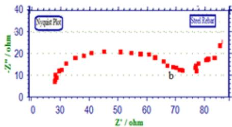
**Fig.2: AC Impedance spectra of rebar steel immersed in (a): SCPS prepared in well water (b): SCPS + 250ppm of PDC+50ppm of Zn<sup>2+</sup> (Nyquist plots)**
