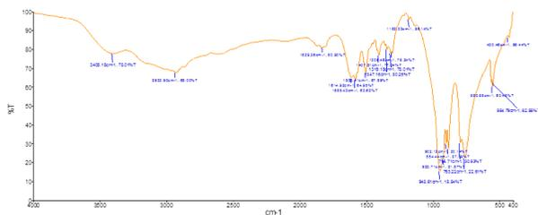
**Fig.5(b): FTIR spectrum of film formed on the metal surface after immersion in aqueous solution containing SCPS + 250 ppm PDC + 50 ppm of  $\text{Zn}^{2+}$**
