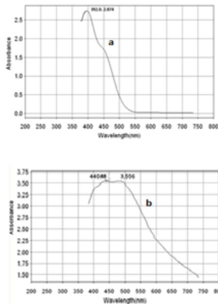
**Fig.4:UV-Visible spectrum of solution containing (a) SCPS + pure PDC (b) SCPS+PDC+Fe<sup>2+</sup>**
